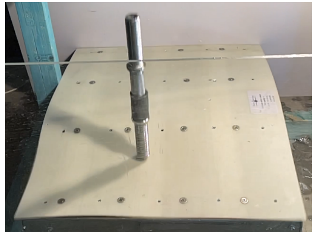
Figure 8: 72.5 J Rock Impact Testing
